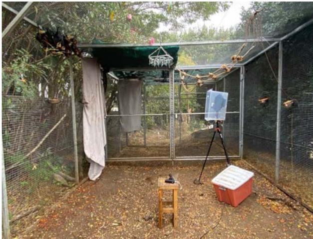
Figure 1. The sound camera mounted on a tripod while recording vocalizations of Mauritian fruit bats (*Pteropus niger*) at Yovel's Bat Lab research station, Mauritius, September 2023.
